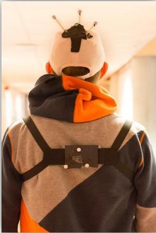
**Figure 5 - Head and back markers used for acquiring ground truth**
