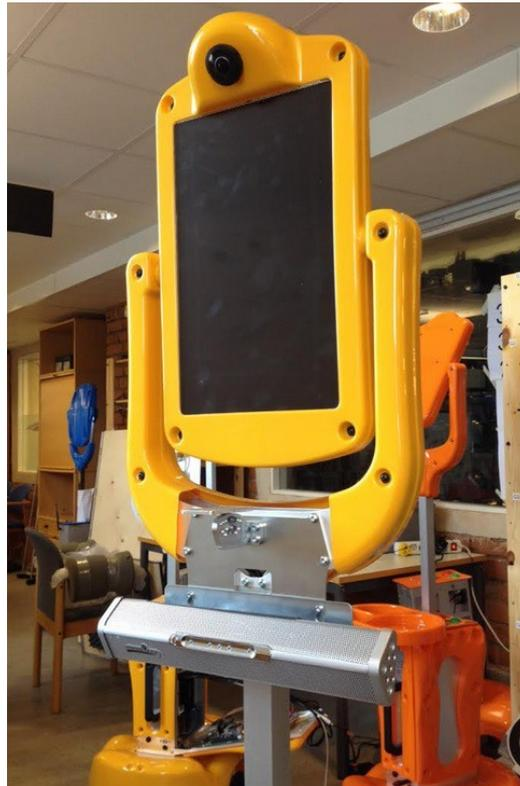
Fig.2 High-Definition camera mount and array microphone
